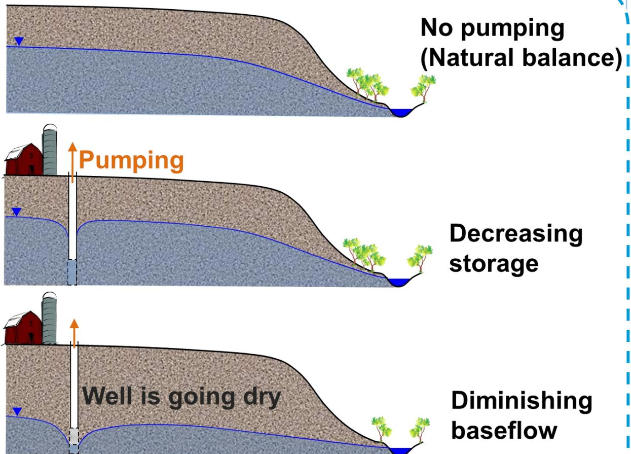
Figure 4: Cross section illustrating the impact of pumping on the water table. The top diagram shows the natural balance (no pumping). As pumping increases (middle) there is a decrease in storage. If pumping continues at an unsustainable rate, the water level drops to a point where the well will be dry and stream baseflow will be impacted.
