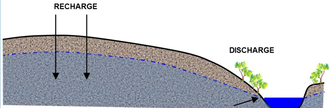
Figure 1: The natural water balance. Recharge - Discharge  $\approx 0$  over the long-term average
