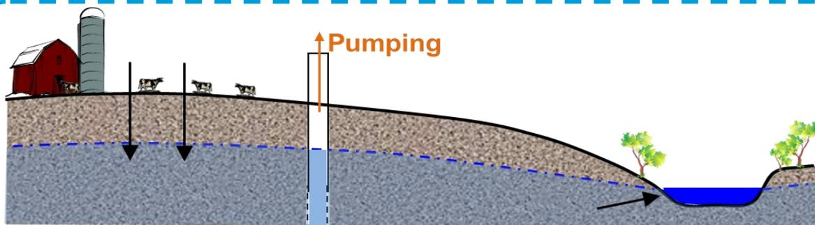
Figure 3: A new water balance with pumping. This new balance occurs when pumping remains smaller than recharge and there is a reduction in the amount of natural discharge.
