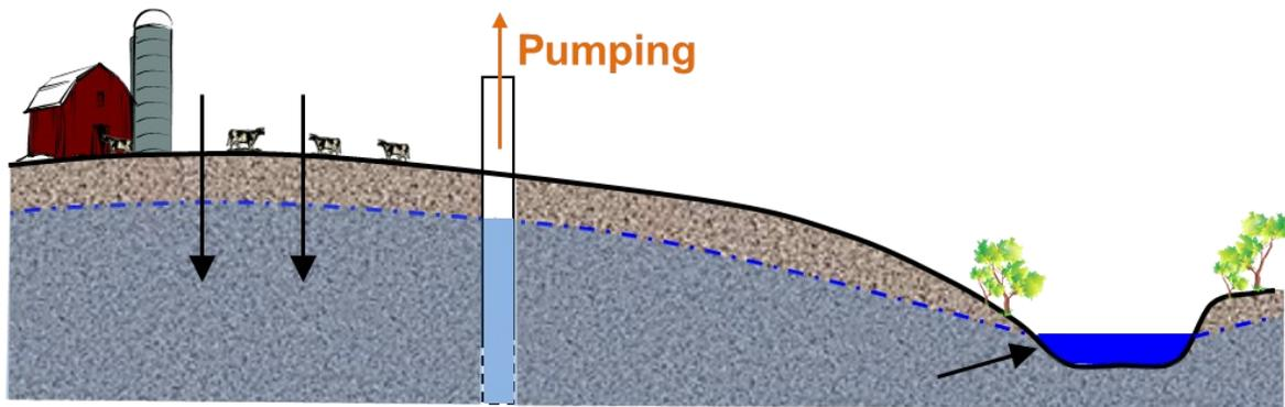
Figure 2: The addition of a well pumping from an aquifer disturbs the water balance.
