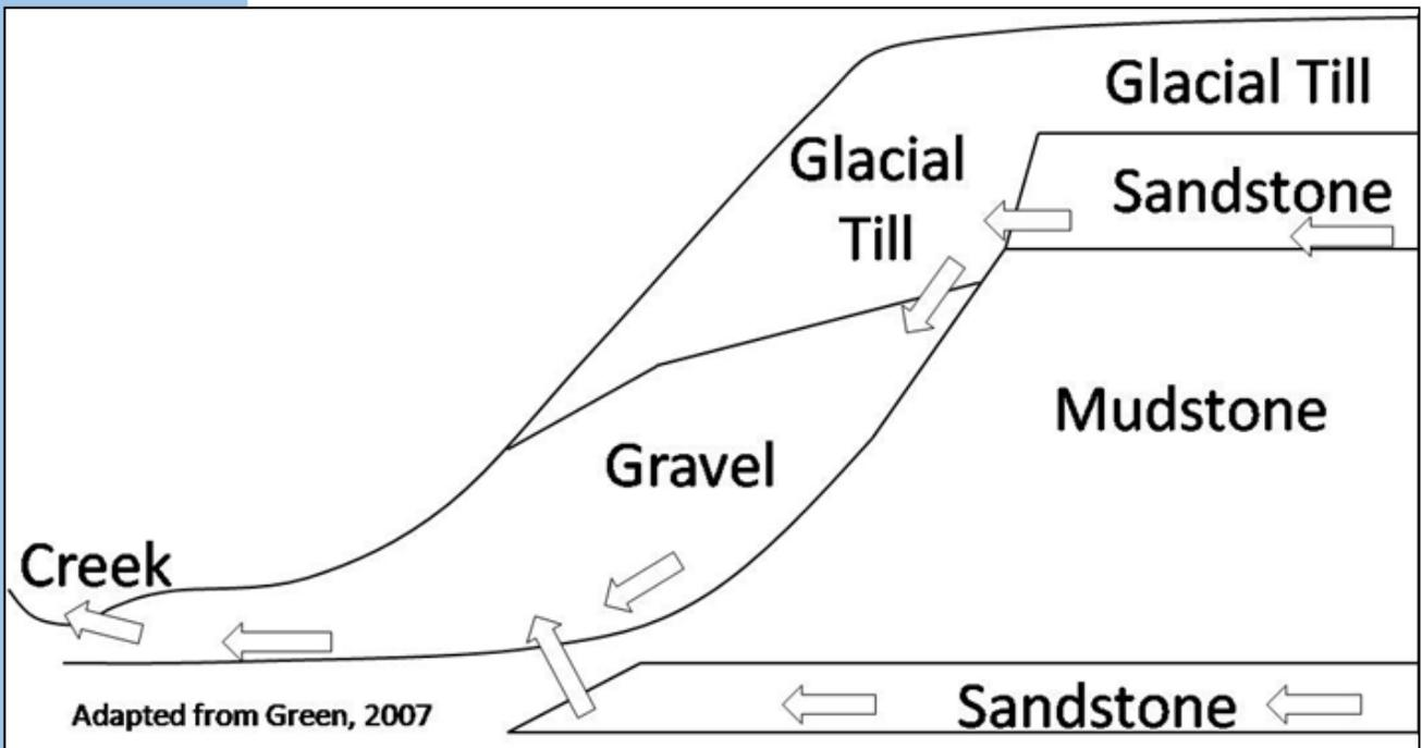
Figure 2b: Alternative geological profile of spring outlet through glacial till and gravel from sandstone layers (Adapted with permission, Green, 2007).
