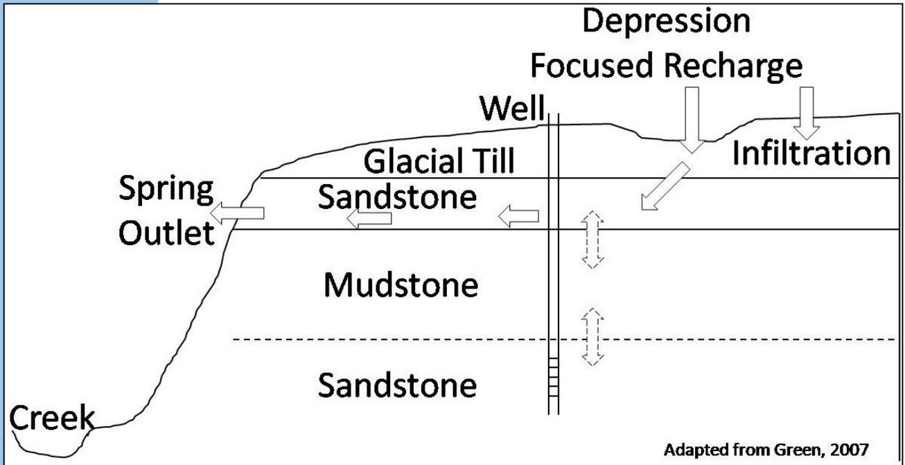
Figure 2a: Typical geological profile of spring outlet from sandstone layer exposed at the edge of a stream channel. Solid arrows indicate groundwater flow; dashed arrows indicate flow to deeper geological layers. (Adapted with permission, Green, 2007).
